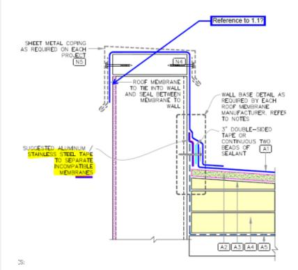
ROOF MEMBRANE MANUFACTURER SHALL PROVIDE A BASE FLASHING DETAIL, WHERE ROOF AIR IS VAPOR BARRIER SHOULD BE EXTENDED VERTICAL UP TO SEAL WITH ROOF MEMBRANE. THIS SETAIL WILL ADDRESS THE MEMBRANE'S MECHANICAL ATTACHMENT AGAINST WIND UPLIFT PRESSURE ALSO.
